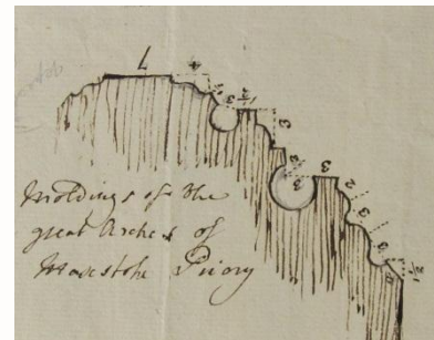
Sketch of mouldings of great arches, with measurements, of Maxstoke Priory
