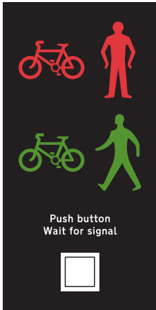
Near-side signals for Toucan crossing
