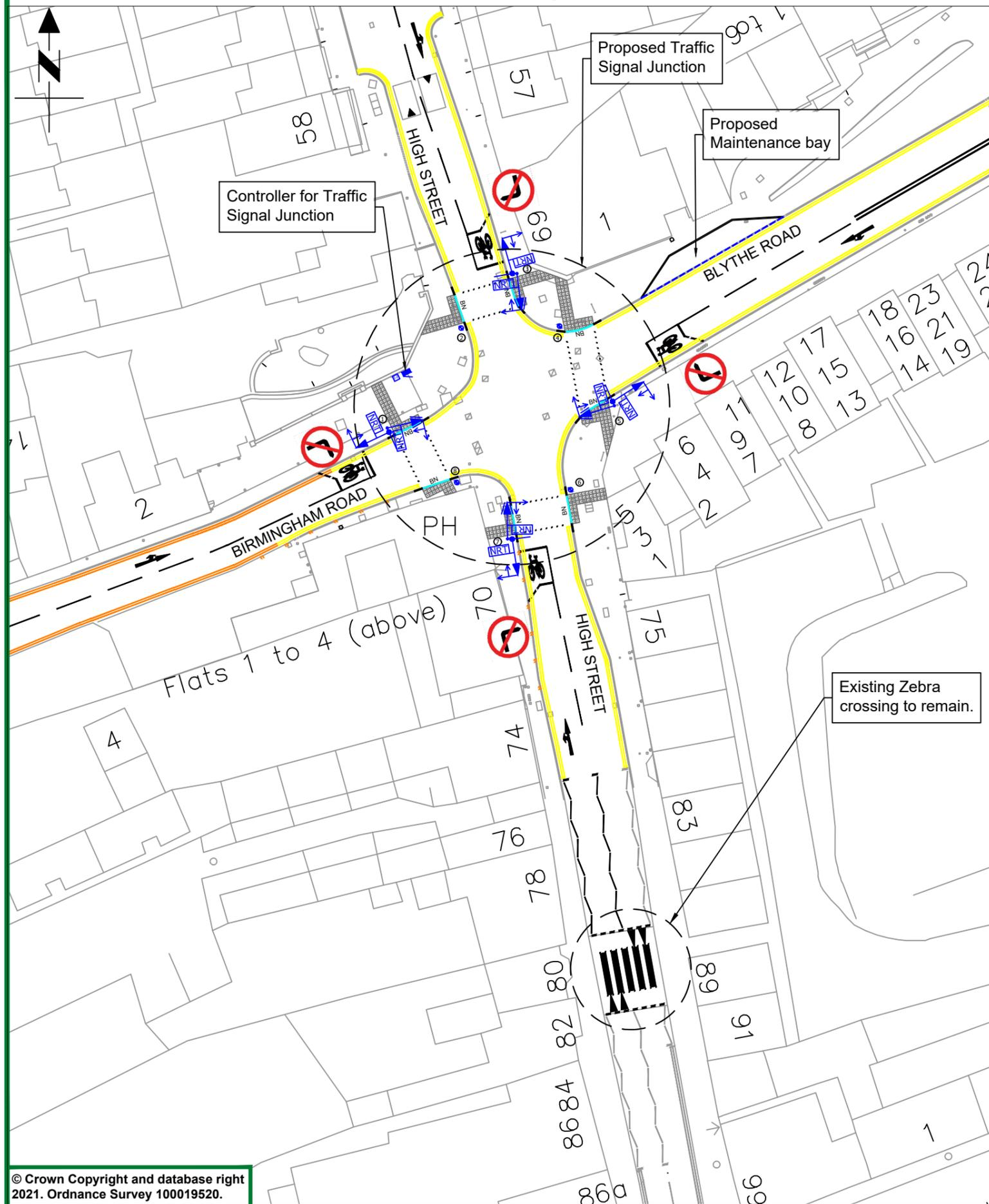
The proposed traffic signal junction will incorporate controlled pedestrian crossing facilities on all four arms of the junction.
