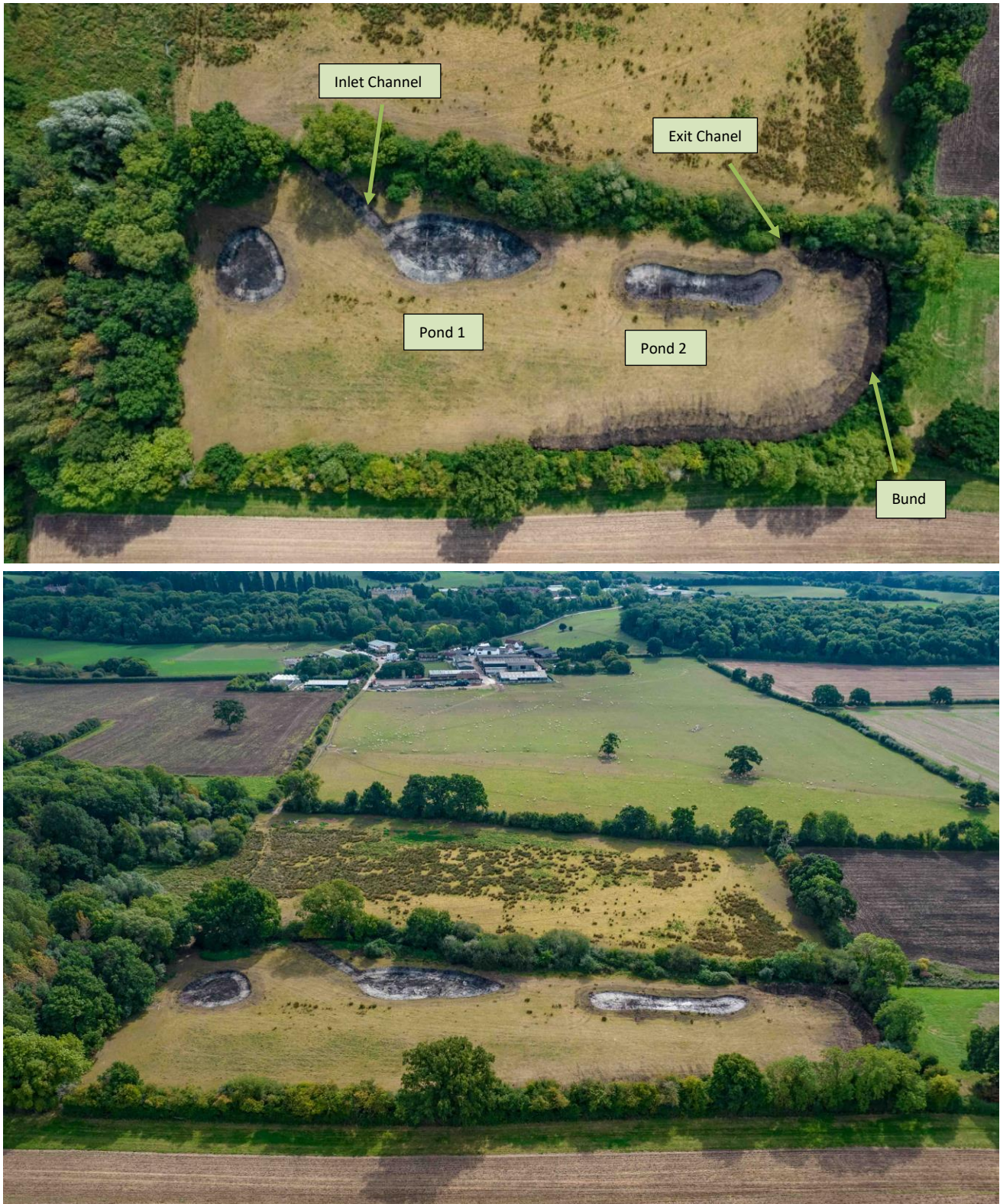
Figure 8 - Images of the Wellesbourne Flood Action Group NFM works approved by WCC.
