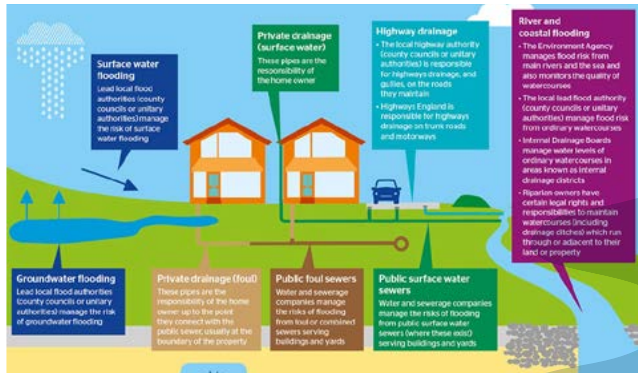
Figure 2: Diagram of possible contributing factors to flooding, and who would be responsible. Source: Southern Water www.southernwater.co.uk/help-advice/flooding/flooding-who-s-responsible
