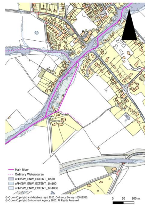
Source: Environment Agency (Risk of Flooding from Surface Water, main river mapping). Note this is modelled information indicative of the main risk areas. It does not indicate the areas that flooded in August 2020. Darker blues indicate higher risk.
