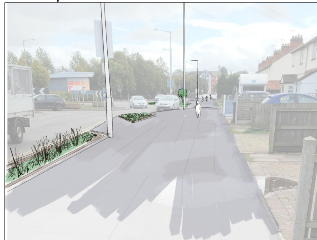
Rain gardens on the edge of pavements to capture surface runoff from roads, slowing down rates of flow, and helping to infiltrate pollutants. The planting also contributes to biodiversity and provides a buffer between vehicles and users of the pavement.
