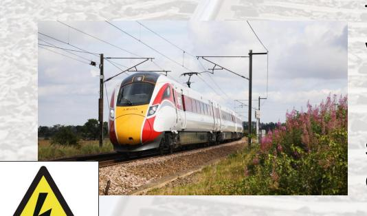
The rail next to the track has 750 volts running through it . Overhead power lines carry 25000 volts - that is 100 times greater than the power supply in your home. The electricity can even jump so you don't necessarily have to touch the live wires and rails to be injured.
