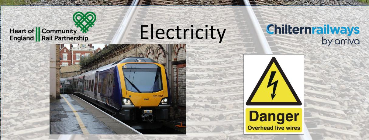
Some trains are powered by electricity. The rail next to the track has 750 volts running through it . Overhead power lines carry 25000 volts – that is 100 times greater than the power supply in your home. Heart of Community England Rail Partnership
